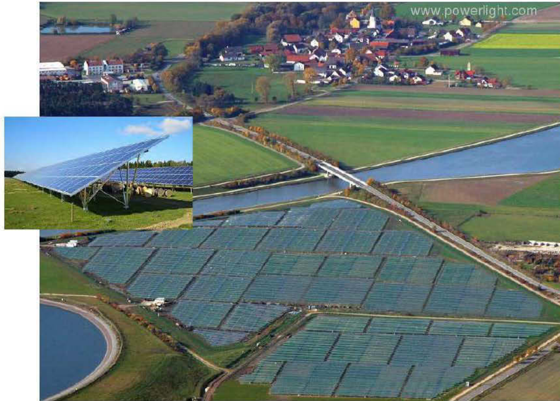
Bavaria Solar Park: 5 \text{ W/m}^2 ; this picture shows 0.7 \text{ MW} (average)
